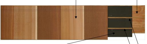
**Galvanized Staples** The cedar is attached with 2 staples at the top of each shingle. Then the panel is flipped over and staples are added through the back to secure the shingle butts while the glue cures
