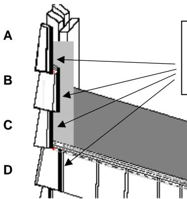
Caulk all butt joints along the cut edge of the panel's backer. Fit snugly against corner or trim.
