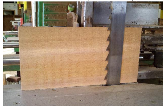
Picture of cross grain sawing of shingles
